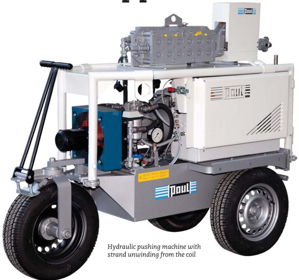
*Hydraulic pushing machine with
